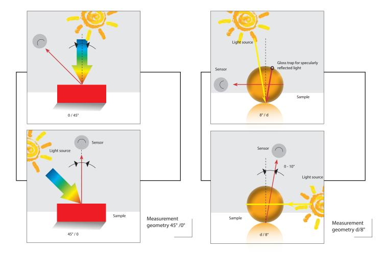
The area of application determines which measurement geometry is used.
