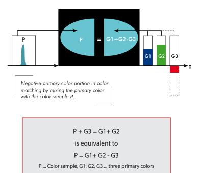
On account of these restrictions, in 1931, the CIE defined three arbitrary imaginary measurement values (X, Y and Z) as primary color stimuli – selected from the point of view of easy colorimetric evaluation. All real colors can be represented by additive mixing using these three measurement values. These measurement values are called 'CIE standard tristimulus values', and the color space is called 'CIE XYZ color space'.
