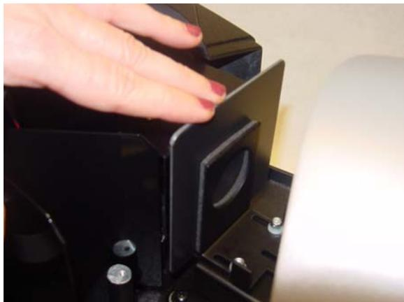
4. When the measurement is completed, remove the black card from the transmission compartment.
