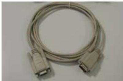
1. Connect the 9-pin male connector on the serial cable to the RS-232C female connector on the rear panel of the instrument.
