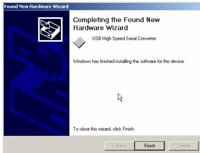
5. Click **Finish**. **Do not remove the USB Driver CD from the system.** The “Found New Hardware Wizard” will automatically appear again, and the process must be repeated a second time to complete the software installation.
