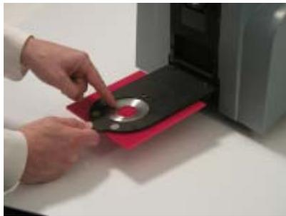
3. The backside of this door reveals the area of the sample covering the port opening. If necessary, adjust the placement of the sample to target the portion of the sample to be measured.
