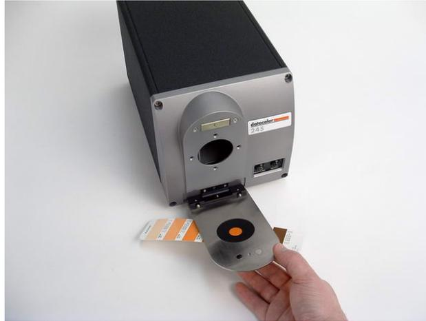
3. If necessary, adjust the placement of the sample to target the portion of the sample to be measured. The sample must completely cover the port opening.
