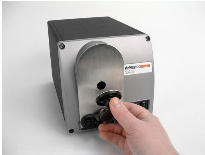
2. Position the sample at the port. The sample should completely cover the port opening.
