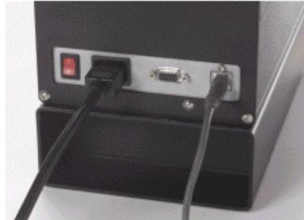
1. Plug the female end of the power cord into the power receptacle on the rear panel of the instrument. Insert the plug into a standard AC outlet.
