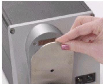
2. Pull top of door down to its full horizontal position. The backside of this door reveals the area of the sample covering the port opening.
