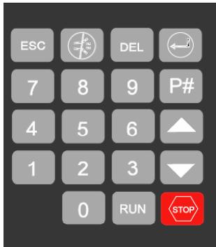
The Ahiba IR numeric keypad is a membrane keypad that contains 19 keys.
