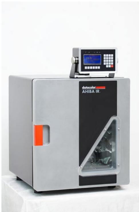
The Ahiba IR controller includes software that is used to program customized temperature/time sequences. Microprocessor technology ensures that the controller accurately follows the pre-defined dyeing curves.
