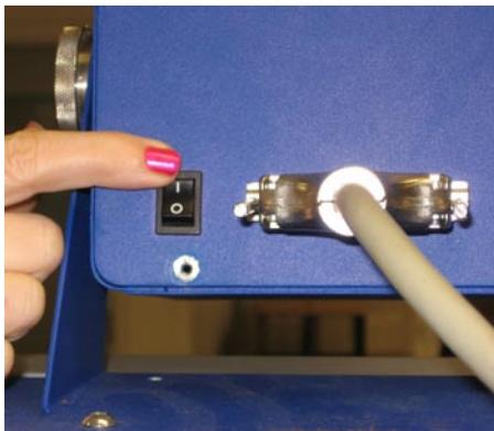
3. Press the top of the button to activate the controller. Press the bottom of the button to cut the power to the controller.
