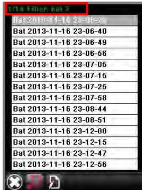
6. Use the *up/down arrow keys* to select a batch from the list, and press **OK**. The data for the batch will display.
