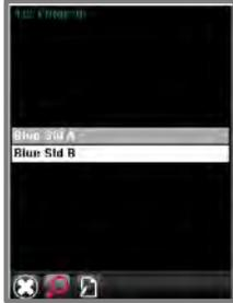
6. Use the *up/down program navigation keys* to select a standard from the list, and press **OK**. The data for the standard will display.
