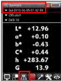
1. After the standard is selected, navigate to the *Batch Editing* icon on the Live Bar and press **OK**.
