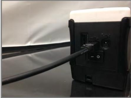
2. Connect the large USB connector on the instrument cable to a USB port on the computer.
