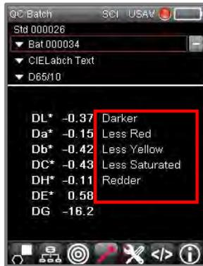
This screen includes color differences *and* text 'descriptors'. The descriptors convert the numerical differences into text descriptors. Depending on the samples in the evaluation, you will see text such as *lighter, redder, bluer*, etc. In this example, the value for Db\* is translated as follows:
