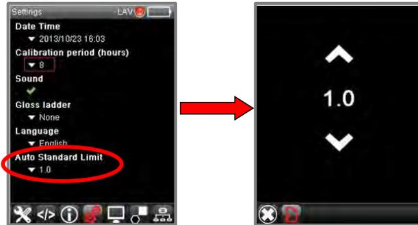
In this example, the program will discard all standards that are more than 1.0 DE CIEL\*a\*b\* from the active batch.
