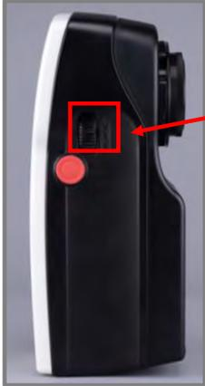
A switch on the side of the instrument next to the Measure button is used to change the lens position on a dual aperture instrument. The device is fitted with a sensor to detect the lens selection on the instrument.
